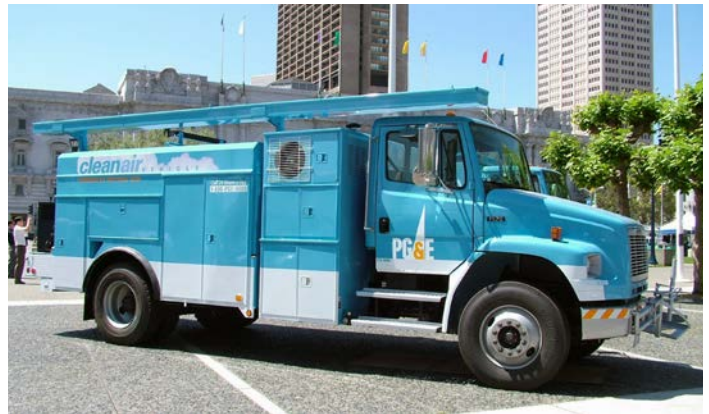
Pacific Gas and Electric chose to convert its heavy-duty trucks to run on natural gas to obtain the emissions benefits and engine performance it was looking for. Photo from Pacific Gas and Electric, NREL 14921
